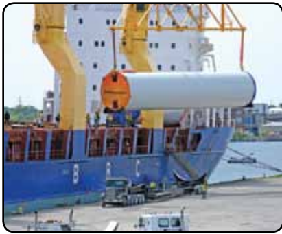
A wind turbine tower section is lowered onto a waiting truck at the port in Menominee, Mich., using the ship's cranes. The truck then moves to the staging area where tower sections are lifted by cranes and stored on the grounds. Photos © Dick Lund.
